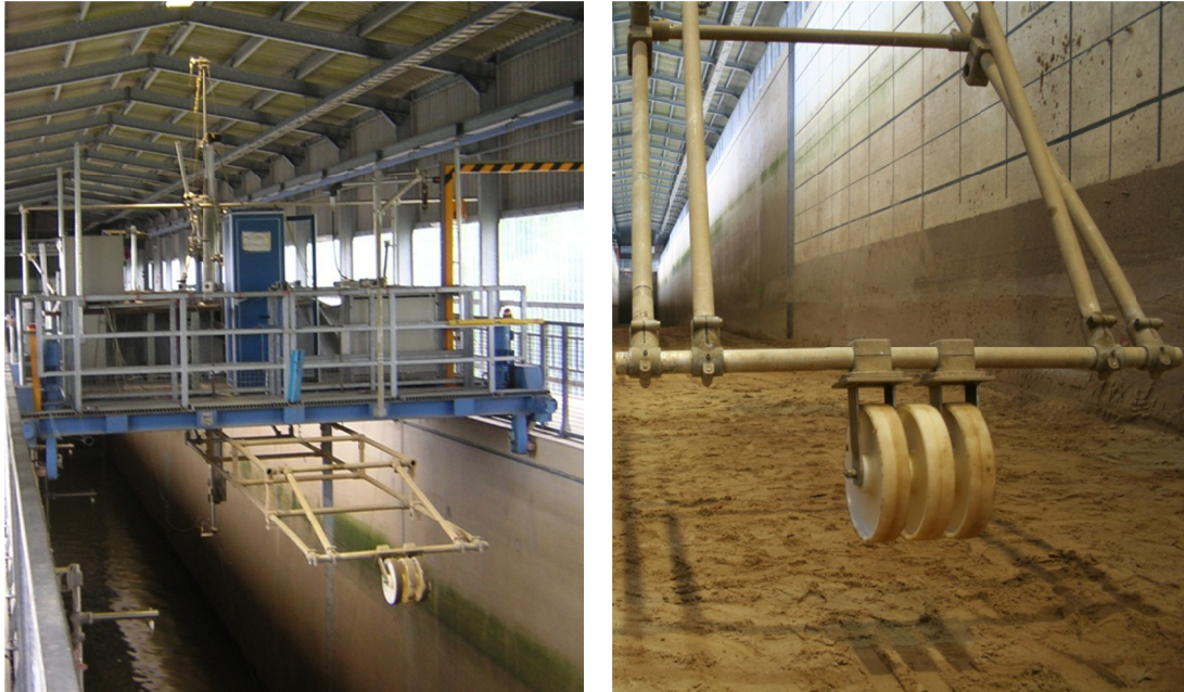
Figure 5.2. Bed profiling wheel of the Large Wave Flume. Fixed on the measurement carriage (left picture) and lowered from the carriage towards the bed (right picture).
