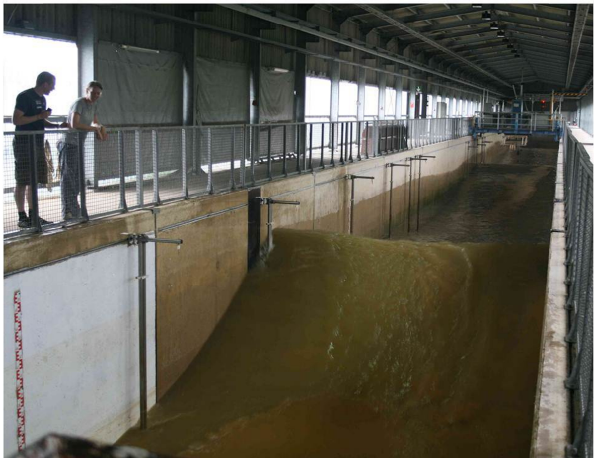
Figure 1.4 Large wave flume (GWK) without water, with measurement frame and mobile sand bed (top left), schematised cross section with dimensions of the sand bed, water depth, wave height and wave boundary layer (top right) and with water and waves (below).
